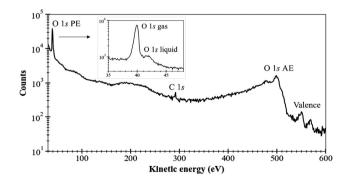
Fig. 3 Total electron spectrum measured on a 1 M sodium benzoate solution with photon energy h $\nu$  = 580 eV, an energy step 1 eV (0.1 eV in the layout), and a count rate of 13k-17k e<sup>-</sup> s<sup>-1</sup> during a recording time of about 1 h, count-rate is given in logarithmic scale. Energy calibration was performed on the O 1s gas signal and Ar 2p resonances
