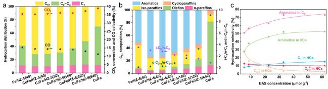
Fig. 2 Hydrocarbon distribution (a) and  $C_{5+}$  composition (b) in the case of  $CO_2$  hydrogenation over various catalysts; (c) effect of the BAS concentration on the performance of composite catalysts. N- $C_{5+}$  means  $C_{5+}$  hydrocarbons other than aromatics.  $C_{2-4}^0$  and  $C_{2-4}$  denote the paraffins and olefins of  $C_2$ - $C_4$  hydrocarbons, respectively. Reaction conditions: 320 °C, 3.0 MPa,  $H_2/CO_2/N_2 = 72/24/4$  (vol%), 4000 mL  $H_2/CO_2/N_2 = 72/24/4$
