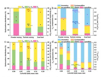
Fig. 3 Hydrocarbon distribution (a) and  $C_{5+}$  composition (b) in the case of  $CO_2$  hydrogenation over CoFe/HZ-5(40) with different proximities; hydrocarbon distribution (c) and  $C_{5+}$  composition (d) of  $CO_2$  hydrogenation over tandem catalysts with different CoFe/HZ-5(40) mass ratios. Reaction conditions:  $320\,^{\circ}C$ ,  $3.0\,$  MPa,  $H_2/CO_2/N_2 = 72/24/4$  (vol%),  $4000\,$  mL  $g_{cat}^{-1}\,h^{-1}$ , time on steam = 14 h.
