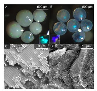
(A) 370PC ⊂ CsPbBr<sub>3</sub> micrographs of  $190PC \subset CsPbCl_{1.5}Br_{1.5}$  microbead hybrids exposed to light from above in silicone oil with insets of hybrids illuminated with  $\lambda_{ex}$  = 365 nm. SEM of (C)  $370PC \subset CsPbBr_3$  and (D)  $190PC \subset CsPbCl_{1.5}Br_{1.5}$ .
