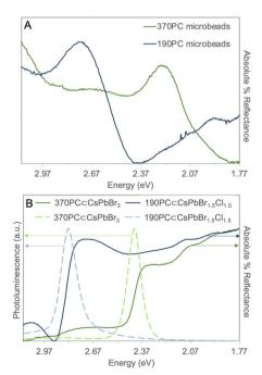
Fig. 1 (A) Absolute % reflectance of 370PC and 190PC microbeads and (B) normalized optical data for 370PC ⊂ CsPbBr<sub>3</sub> and 190PC ⊂ CsPbBr<sub>1.5</sub>Cl<sub>1.5</sub> hybrids ( $\lambda_{ex} = 365 \text{ nm}$ ).
