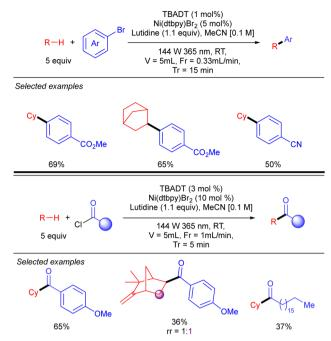
Scheme 29 Ni/TBADT-catalysed arvlation and acylation of simple alkanes under flow chemistry conditions.
