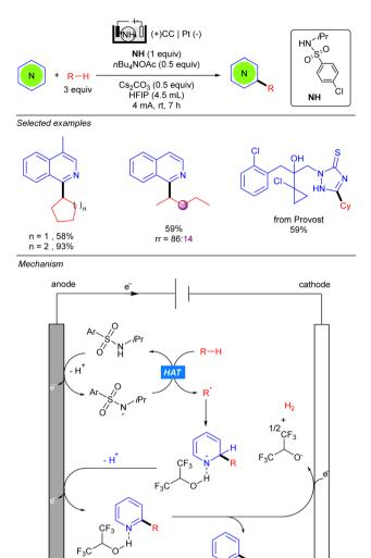
Scheme 43 Electrochemical alkylation of nitrogen heterocycles using an N-alkyl sulfonamide as the HAT reagent.
