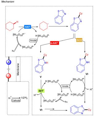
Scheme 44 TBADT-catalysed photoelectrochemical alkylation benzothiazoles.
