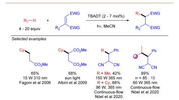
Scheme 22 TBADT-catalysed radical conjugate addition of alkanes.
