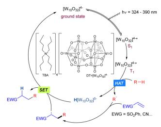
Scheme 21 General photocatalytic action mechanism of TBADT.
