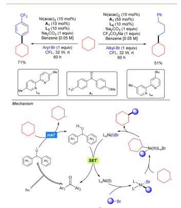
Scheme 39 Ni/ketone-catalysed C(sp<sup>3</sup>)-H arylation and alkylation of alkanes
