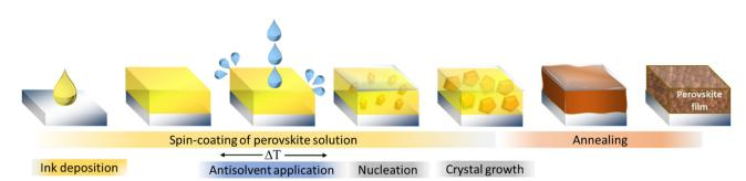
Fig. 1 Schematic illustration of the fabrication of metal halide perovskite layers by the solvent-engineering method
