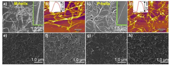
Fig. 2 SEM and AFM images of supramolecular structures of (a and b) Ag<sup>+</sup>-L-1 formed in THF, and (c-h) Ag<sup>+</sup>-D-1 in (c and d) THF, (e) EtOH. (f) MeOH. (q) CH<sub>3</sub>CN and (h) H<sub>2</sub>O. The insets in (a) and (c) show, respectively, two types of polymeric structures, namely the M-helix of  $Aq^+-L^-1$  and P-helix of  $Aq^+$ D-1.  $[Ag^+-L-1] = [Ag^+-D-1] = 25 \mu M$ .
