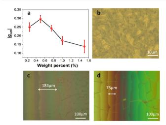
Fig. 2 (a) The tendency of CPL  $g_{\rm lum}$  values with different mixing weight ratios of R-1-C,  $\lambda_{\rm ex}$  = 360 nm, all error bars show the mean  $\pm$  standard deviation, n = 5 independent experiments. (b) POM image of R-1-C/E7, [R-1-C] = 0.5 wt%. POM images of N\*-LC including 0.5 wt% (c) R-1-O and (d) R-1-C in wedge-shaped cells at room temperature.
