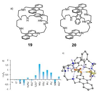
Fig. 8 (a) Structures of receptors **19** and **20**. (b) Fluorescence response of **19** measured in the presence of 200 equiv. of anions (50 mM acetate buffer, 5% DMSO, pH 3.6. (c) Molecular structure of the nitrate complex  $\mathbf{19H_6}^{6+}(NO_3^-)(CH_3OH)$  according to the X-ray analysis. Adapted with permission from ref. 42. Copyright 2019 American Chemical Society.
