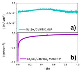
Fig. 4 CPP at 0 V vs. RHE of the hybrid photocathodes Sb<sub>2</sub>Se<sub>3</sub>/CdS/TiO<sub>2</sub>/ NiP (a) and Sb<sub>2</sub>Se<sub>3</sub>/CdS/TiO<sub>2</sub>-meso/NiP (b) in 0.1 M Na<sub>2</sub>SO<sub>4</sub> pH 3 at 100 mW cm<sup>-2</sup> and  $\lambda > 340$  nm.
