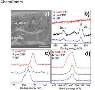
Fig. 3 (a) Cross-sectional SEM image of Sb<sub>2</sub>Se<sub>3</sub>/CdS/TiO<sub>2</sub>-meso/NiP. (b-d) XPS spectra of NiP molecular catalyst (blue trace) after it is immobilized on TiO2 (pre-CPP,black trace), and after 5 h of CPP test at 0 V vs. NHE (post-CPP, red trace) with light intensity of 100 mW cm<sup>-2</sup> and  $\lambda > 340$  nm in 0.1 M Na<sub>2</sub>SO<sub>4</sub> at pH 3. (b-d) XPS spectra showing Ni 2p, P 2p and N 1s regions respectively.
