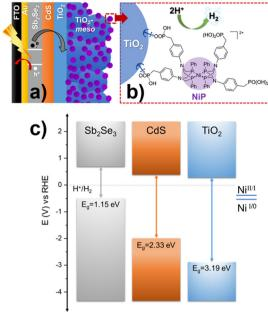
Fig. 1 (a) Schematic diagram of Sb<sub>2</sub>Se<sub>3</sub>/CdS/TiO<sub>2</sub>-meso/NiP hybrid photocathode. (b) Chemical structure of NiP catalyst molecular catalyst, panel a and b are not drawn to scale. (c) Equilibrium band alignment diagram of  $Sb_2Se_3/CdS/TiO_2$  heterojunction based on  $VBM^{11}$  and  $E_0$ measured separately for each layer (Fig. S2.1, ESI†), note that NiP redox couple is pH independent.21
