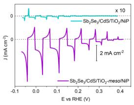
Fig. 2 Chopped light LSV of the hybrid photocathodes Sb<sub>2</sub>Se<sub>3</sub>/CdS/TiO<sub>2</sub>/ NiP (blue trace) and Sb<sub>2</sub>Se<sub>3</sub>/CdS/TiO<sub>2</sub>-meso/NiP (purple trace) at 10 mV s<sup>-1</sup>. The TiO<sub>2</sub>-meso enables a higher loading of the **NiP** catalysts and increased photocurrents. All experiments were carried out in 0.1 M  $Na_2SO_4$  pH 3 at 100 mW cm<sup>-2</sup> and  $\lambda > 340$  nm.
