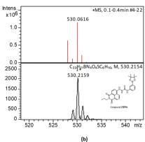
Fig. 2 HR mass spectrometry (ESI<sup>+</sup>) and best fit isotopes match found at the analysis of compounds **1-Bpin** (a) and compound **2-Bpin** (b). The compound fragmentation and loss of pinacol group/deprotection was typically being observed during LC-MS ESI<sup>+</sup> analysis of all compounds in this series. Further mass spectrometry data are given in ESI.†
