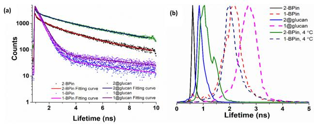
Fig. 9 TCSPC and 2P FLIM comparisons: (a) overall TCSPC decay curves for compounds in DMSO, two-photon  $\lambda_{ex}$  910 nm: (a) 2P TCSPC for compounds **1-BPin** 1@β-p-glucan, **2-BPin**, 2@β-p-glucan where compounds **1-BPin** and **2-BPin** were each incubated in presence of excess beta-p-glucan forming **1**@β-p-glucan and 2@β-p-glucan, respectively *in situ*. (b) Overall lifetime distribution of compounds in cells, multiphoton  $\lambda_{ex}$  = 910 nm. Fitted data are given in ESI.†
