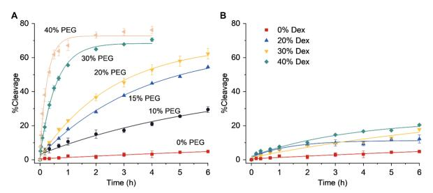
Fig. 2 Effect of molecular crowding on DNAzyme activity. The dependence of the DNAzyme activity on the amount of (A) PEG or (B) Dex. Error bars were derived from two independent experiments.
