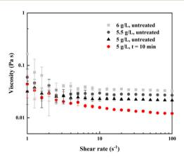
**Fig. 2** Viscosity profiles of untreated and 10 min-treated alginate solutions. In grey are reported the data for control solutions with higher concentrations (5.5 and 6 g L<sup>-1</sup>) to show the effect of water evaporation. Data are expressed as average  $\pm$  standard deviation; n = 3.
