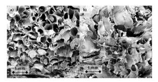
Fig. 3 Representative SEM images of the fracture of untreated (a) and 10 min NTP-treated (b) cross-linked alginate from 5 g L<sup>-1</sup> alginate solutions.
