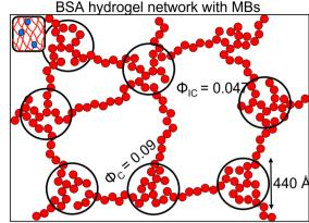
Fig. 7 Predicted structure of the BSA hydrogel network Left in the absence of MBs and Right in the presence of MBs. The smaller red and blue circles represent folded proteins, the black circles represent the fractal-like clusters ( $\phi_C$ ) connected with proteins in the inter-cluster space ( $\phi_{IC}$ ).
