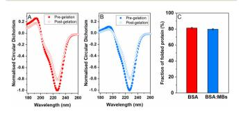
Fig. 4 Normalized circular dichroism spectra of BSA for (A) the standard BSA gel and (B) BSA: MB gel at a MB concentration of 109 MB per mL, with spectra included for both before gelation (squares) and postgelation (circles). (C) Comparison of the peak at 222 nm associated with the  $\alpha$ -helical structure of BSA.
