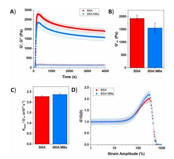
Fig. 5 (A) Gelation curve show the storage (filled) and loss moduli (hollow) over time for control BSA hydrogel in the absence (red squares) and presence (blue circles) of MBs. (B) Relaxed storage modulus  $(G'_{\infty})$ from fitting eqn (1) and (C) kinetic parameters,  $k_{\text{max}}$ , normalized to  $G'_{\infty}$  with changing the MB concentration. (D) Non-linear behaviour of BSA hydrogels in the absence (red squares) and presence (blue circles) of MBs.
