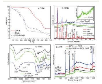
Fig. 7 Different characterisation methods used to provide support to the successful synthesis of ZIF-8/PAM hybrid. (a) TGA, (b) powder XRD, (c) FT-IR, (d) XPS. Reproduced from ref. 63 with permission from John Wiley and Sons, copyright 2019.
