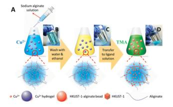
Fig. 5 (A) Schematic of the preparation of the MOF-alginate composite. Photographs of (B) alginate hydrogels cross-linked to Cu<sup>2+</sup>, (C) alginate metal hydrogels after washing, (D) MOF-hydrogel hybrids. Reprinted with permission from ref. 62. Copyright 2016 American Chemical Society.
