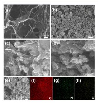
**Fig. 6** SEM images of (a) Graphene hydrogel (b) cZIF-8 (c) MOF-hydrogel (d) Quantum dots on MOF-hydrogel. (e-h) Elemental mapping of the Quantum dots on MOF-hydrogel. Reproduced with permission from ref. 72. Copyright 2020 Elseiver.
