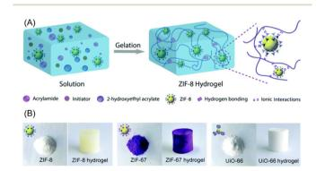
Fig. 2 (A) Synthetic strategy of adding the MOFs to a pre-polymer solution with the required monomers and initiators. Gelation gave the MOFhydrogel hybrid. (B) The MOF powders and composite MOF-hydrogels as synthesized. Reproduced from ref. 32 with permission from the Royal Society of Chemistry, copyright 2019.
