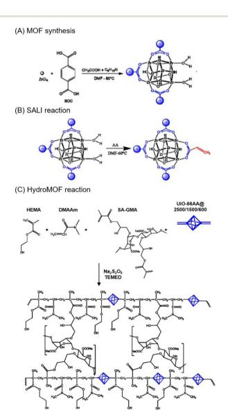
Fig. 4 Schematic showing the mechanism of the MOF-hydrogel. (a) Preparation of UiO-66 MOFs (b) Reaction of SALI in DMF to functionalise the UiO-66. (c) Formation of the hydroMOF using a radical polymerisation reaction. Reproduced with permission from ref. 60. Copyright 2021 Elsevier.
