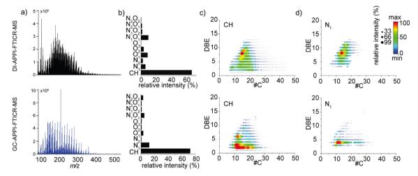
Fig. 1 (a) Mass spectra of plastic pyrolysis oil obtained for DI-APPI-FTICR MS (at the top) and average mass spectra over 0 to 80 min obtained for GC-APPI-FTICR MS with toluene as dopant (at the bottom) with their (b) molecular classes distribution, (c) DBE *versus* carbon number plot of CH class, and (d) DBE *versus* carbon number plot of  $N_1$  class.
