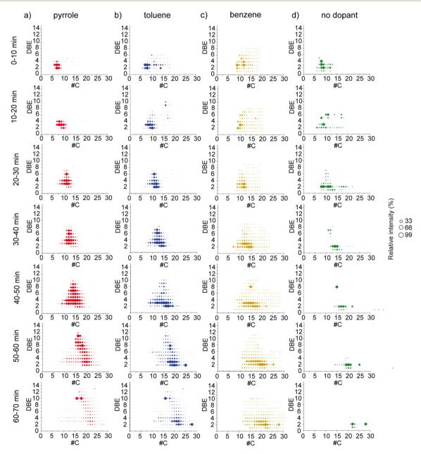
Fig. 5 DBE *versus* carbon number plots of CH class for plastic pyrolysis oil for seven retention time segments of GC-APPI-FTICR MS experiments with (a) pyrrole (red), (b) toluene (blue), (c) benzene (yellow), and (d) no dopant (green) for the CH class. The relative intensity was normalized for each DBE *versus* the carbon number plot.
