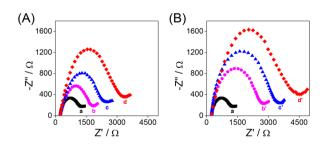
Fig. 1 Nyquist plots of different modified QCM Au chips in 5 mM [Fe  $(CN)_6 I^{3-/4-}$  (1:1) solution containing 0.1 M KCl (frequency,  $10^5-0.1$  Hz). (A) (a) Bare Au chip, (b) aptamer/Au chip, (c) BSA/aptamer/Au chip, and (d) RBD/BSA/aptamer/Au chip; (B) (a) bare Au chip, (b') antibody/Au chip, (c') BSA/antibody/Au chip, and (d') RBD/BSA/antibody/Au chip.  $C_{RBD}$  =
