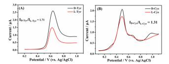
Fig. 11 Differential pulse voltammograms of the Taniaphos– $Cu^+/GCE$  after incubation in 0.1 M PBS containing 1.0 mM  $_{L-/D}$ –Tyr (A) and 1.0 mM  $_{L-/D}$ –Cys (B).
