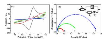
**Fig. 6** Cyclic voltammograms (A) and Nyquist plots (B) of an unmodified GCE (a),  $[(CH_3CN)_4Cu]PF_6/GCE$  (b), Taniaphos/GCE (c) and Taniaphos–Cu<sup>+</sup>/GCE (d) in 0.1 M KCl containing 5 mM  $[Fe(CN)_6]^{4-/3-}$ . Inset of (B): the equivalent circuit, where  $R_s$ ,  $R_{ct}$ ,  $W_d$  and Q represent the solution resistance, charge transfer resistance, Warburg resistance and constant phase elements, respectively.
