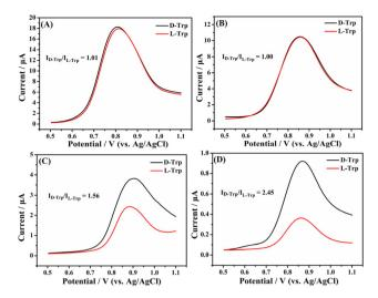
Fig. 7 Differential pulse voltammograms of an unmodified GCE (A),  $[(CH_3CN)_4Cu]PF_6/GCE$  (B), Taniaphos/GCE (C) and Taniaphos-Cu<sup>+</sup>/GCE (D) after incubation in 0.1 M PBS containing 1.0 mM L-Trp and D-Trp.
