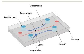
Fig. 3 The general structure of a microfluidic chip.
