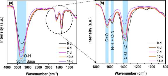
Fig. 4 FTIR spectra of the different chitosan–KOH gel electrolytes prepared with solutions at different ageing days: (a) spectra from 4000 to 700 cm<sup>-1</sup> and (b) magnified views of the spectra from 1800 to 800 cm<sup>-1</sup>.
