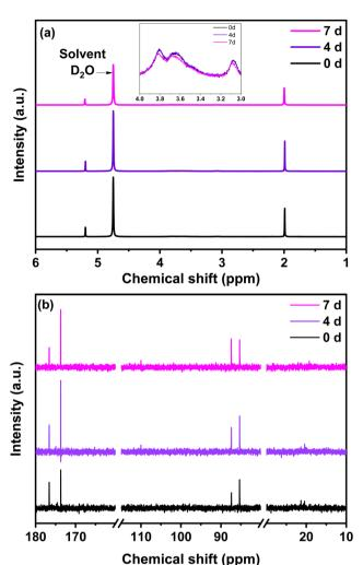
Fig. 3 (a) <sup>1</sup>H NMR (inset: <sup>1</sup>H NMR from 3-4 ppm) (b) <sup>13</sup>C liquid NMR of the chitosan solution at different ageing days, i.e., 0, 4 and 7 days.
