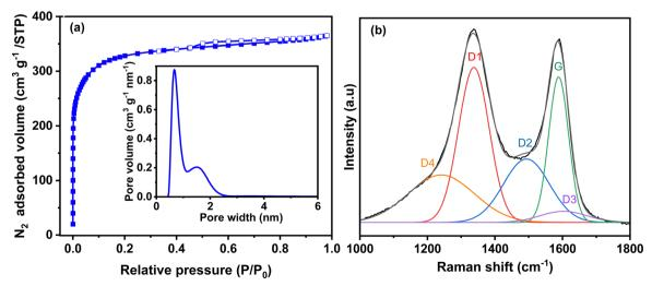
Fig. 2 (a)  $N_2$  adsorption/desorption isotherm (inset: pore size distribution calculated from the 2D-NLDFT heterogeneous surface carbon model for  $N_2$  adsorption) and (b) deconvoluted Raman spectrum of activated carbon Norit R3 Extra. The description of each peak contribution is provided elsewhere.
