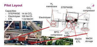
Fig. 21 Layout of the FReSMe project.<sup>89</sup>
