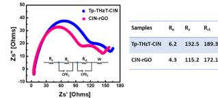
Fig. 7 Impedance plots of the samples Tp-THzT-CIN and CIN-rGO. The model used to fit the impedance is shown in the plot. In the model,  $R_{\rm e}$  corresponds to electrolyte resistance,  $R_{\rm s}$  corresponds to SEI film resistance, CPE1 is the constant phase element of the SEI film,  $R_{\rm ct}$  is charge transfer resistance and CPE2 is the constant phase element for charge transfer.
