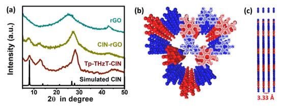
Fig. 1 (a) PXRD patterns of rGO, Tp-THzT-CIN and the CIN-rGO composite compared with a theoretical XRD pattern from a geometrically optimized AA stacked model structure. Top (b) and side view (c) of the space-filled model with ideal eclipsed (AA) packing.
