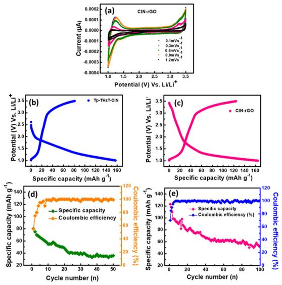
Fig. 6 (a) Cyclic voltammograms of CIN-rGO cycled at different scan rates of 0.1, 0.3, 0.6, 0.9 and 1.2 mV s<sup>-1</sup> between 1–3.5 V. Initial charge discharge curves at 50 mA  $\rm g^{-1}$  current density of Tp-THzT-CIN (b) and CIN-rGO (c). Cycling performance test at 50 mA  $\rm g^{-1}$  current density of Tp-THzT-CIN (d) and CIN-rGO (e).
