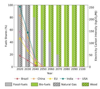
Fig. 1 Transition of the worldwide economy towards net-zero. Following a decreasing carbon intensity (as projected by the IPCC P2 scenario), <sup>6,7</sup> the electricity system becomes carbon neutral in 2050. Fossil-fuels (i.e., diesel and petrol) are progressively replaced by 100% bio-fuels (i.e., bio-diesel and bio-ethanol) in 2080. Natural gas is switched to 100% wood as early as 2040 for biomass drying for BECCS.
