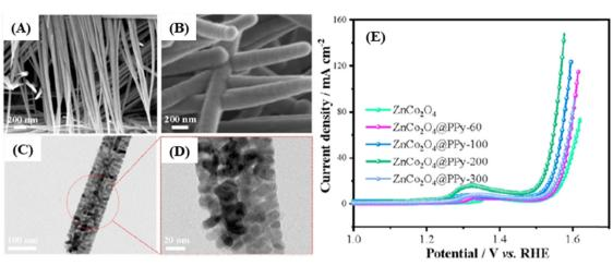
Fig. 21 SEM images of  $ZnCo_2O_4$  (A) and  $ZnCo_2O_4$  (PPy-200 (B). TEM images of  $ZnCo_2O_4$  (PPy-200 (C and D). Linear sweep voltammetry at 2 mV s<sup>-1</sup> for ZnCo<sub>2</sub>O<sub>4</sub> and ZnCo<sub>2</sub>O<sub>4</sub>@PPy samples (E). Reproduced with permission. <sup>275</sup> Copyright © 2021 Elsevier Ltd. All rights reserved.
