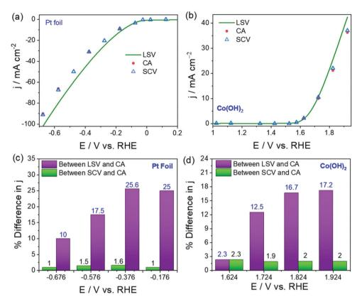
Fig. 4 (a) HER polarization curves of Pt foil acquired using LSV and SCV and provided in comparison with CA data. (b) OER polarization curves of Co(OH)<sub>2</sub> acquired using LSV and SCV and provided in comparison with CA data. (c and d) The plots of % difference in j between LSV and CA, and SCV and CA against potential showing the closeness of SCV and CA. Reproduced from ref. 64 (Copyright 2022, IOP Publishing)
