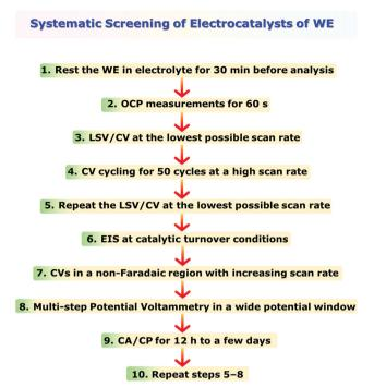
Scheme 2 Systematic use of electroanalytical techniques in assessing a single working electrode for water electrolysis and still getting all the essential information to provide pre- and post-stability and activity
