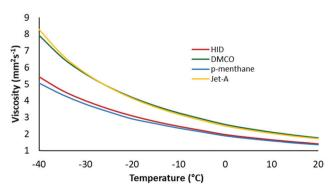
Fig. 3 Kinematic viscosities of HID, DMCO, p-menthane and Jet-A.
