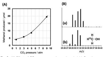
**Fig. 6** (A) Effect of CO<sub>2</sub> pressure on the methanol yield. Reaction conditions: powdered silicon wafer (5 mmol; diameter < 20 μm), CO<sub>2</sub>, H<sub>2</sub>O (10 mmol), TBAF-3H<sub>2</sub>O (0.85 mmol), DMSO (2 mL), 95 °C, 24 h. Yield was determined by GC-FID using an internal standard technique. (B) Mass spectra of methanol produced in the reactions using (a)  $^{13}$ CO<sub>2</sub> and (b)  $^{12}$ CO<sub>2</sub>.
