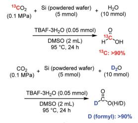
Scheme 1 Isotopic experiment. <sup>13</sup>CO<sub>2</sub>: powdered silicon wafer (5 mmol; diameter  $< 20 \mu m$ ),  $^{13}CO_2$  (1 atm),  $H_2O$  (10 mmol), TBAF-3 $H_2O$ (0.05 mmol), DMSO (2 mL), 95 °C, 24 h. D2O: powdered silicon wafer (5 mmol; diameter  $< 20 \mu m$ ), CO<sub>2</sub> (1 atm, balloon), D<sub>2</sub>O (10 mmol), TBAF-3H<sub>2</sub>O (0.05 mmol), DMSO (2 mL), 95 °C, 24 h.
