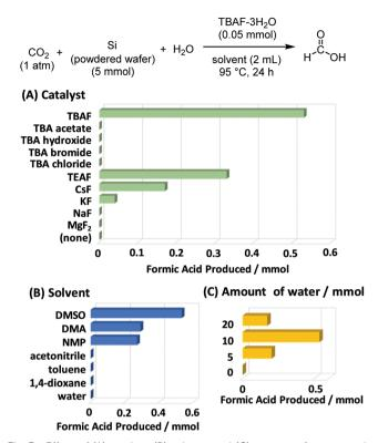
Fig. 3 Effect of (A) catalyst, (B) solvent, and (C) amount of water on the reduction of CO<sub>2</sub> with silicon wafer. Basic reaction conditions: powdered silicon wafer (diameter < 40  $\mu$ m; 5 mmol), CO<sub>2</sub> (0.1 MPa, balloon), H<sub>2</sub>O (10 mmol), TBAF-3H<sub>2</sub>O (0.05 mmol), DMSO (2 mL), 95 °C, 24 h. Yield was determined through internal standard technique of <sup>1</sup>H NMR with CDCl<sub>3</sub> as the solvent and 1,3,5-triisopropylbenzene as the internal standard
