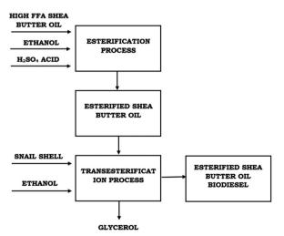
Fig. 2 Flowchart of the two-step acid catalyzed transesterification process
