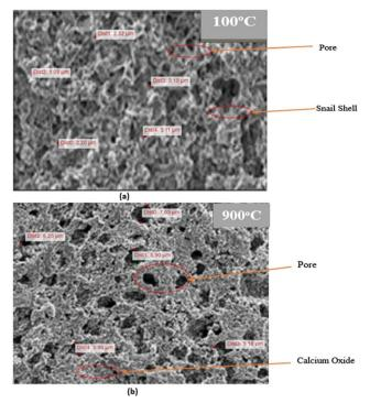
Fig. 5 (a) SEM analysis of the snail shell oven-dried at  $100 \, ^{\circ}\text{C}$  and (b) SEM analysis of the snail shell calcined at 900 °C.
