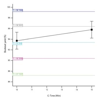
Fig. 12 Effect of reaction time on the shea butter biodiesel yield.
