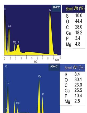
Fig. 6 (a) EDS analysis of the snail shell oven-dried at 100 °C and (b) EDS analysis of the snail shell calcined at 900 °C.
