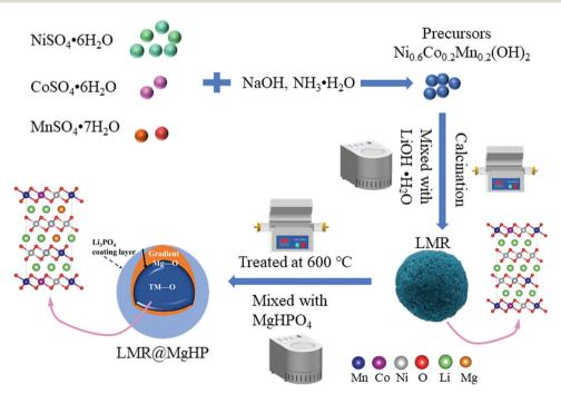
Fig. 1 Scheme of the preparation of LMR@MgHP.
