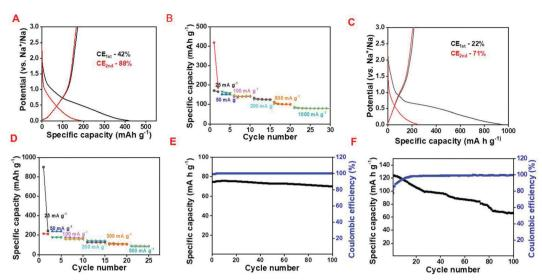
Fig. 7 Half-cell electrochemical study as a Na-ion battery; (A) galvanostatic charge-discharge curve and (B) rate capability curve of NAC, (C) galvanostatic charge-discharge curve and (D) rate capability curve of C/SnO<sub>2</sub>, cycling stability curve of (E) NAC at 1000 mA  $g^{-1}$  and (F) C/SnO<sub>2</sub> at  $200 \text{ mA g}^{-1}$ .
