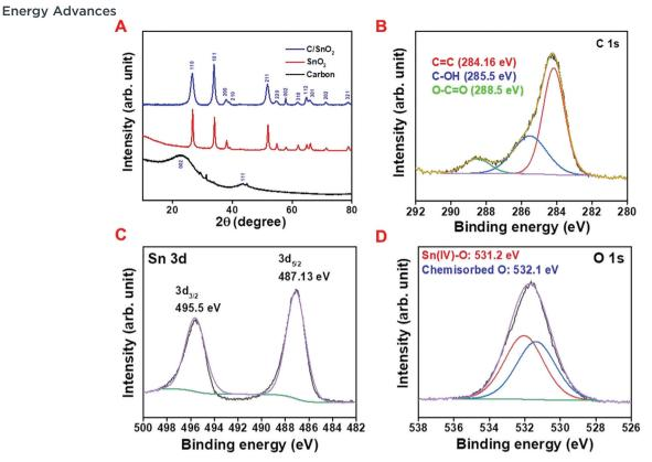
Fig. 2 (A) Comparative X-ray diffraction pattern of NAC (black line), bare SnO<sub>2</sub> (red line) and C/SnO<sub>2</sub> (blue line), X-ray photo electron spectroscopy of the C/SnO<sub>2</sub> composite; (B) C 1s, (C) Sn 3d and (D) O 1s.
