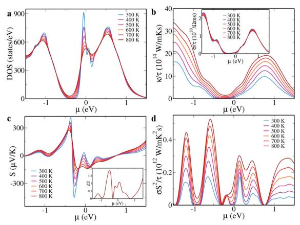
Fig. 2 (a) DOS; (b) thermal conductivity (inset: electrical conductivity); (c) Seebeck co-efficient (inset: ZT@800 K) and (d) power factor of Sn<sub>15</sub>MoTe<sub>16</sub> as functions of chemical potential ( $\mu$ ) at various temperatures. Conductivity and power factor values are reported by scaling them with  $\tau$ .
