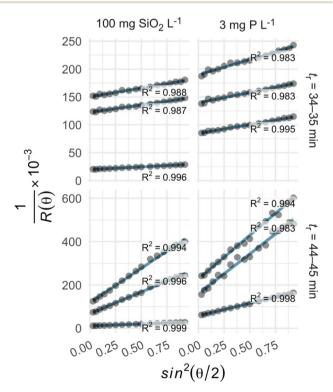
Fig. 1 The Zimm model described the variation in light scattering over the selected range of scattering angles, with  $r^2$  values of 0.983–0.999 (row labels:  $t_r$  denotes retention time).
