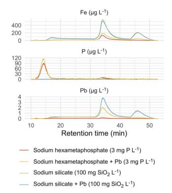
Fig. 4 Fractograms representing sodium silicate and hexametaphosphate suspensions; each is paired with an equivalent suspension dosed with 200  $\mu$ g Pb L $^{-1}$ . Light scattering and absorbance fractograms are displayed with the raw detector responses on the y-axis.
