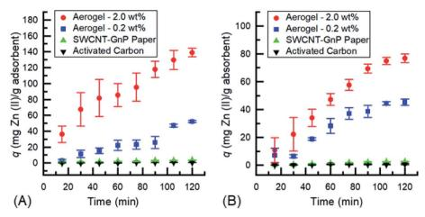
Fig. 4 Time dependent adsorption for removal of adsorbate (Zn(u)) with initial concentrations of (A) 0.5 mg mL<sup>-1</sup> and (B) 0.1 mg mL<sup>-1</sup> by carbon nanomaterial (CNM)-based aerogels of (●) 2.0 wt% and (■) 0.2 wt%, (▲) SWCNT-GnP paper, and (▼) activated carbon
