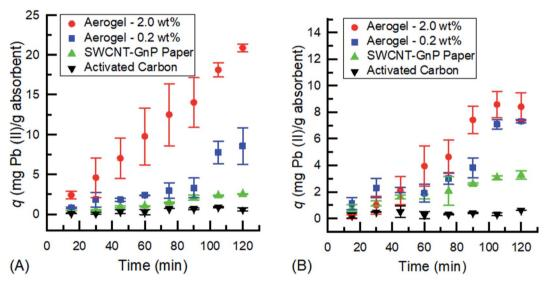
Fig. 5 Time dependent adsorption for removal of adsorbate (Pb( $\parallel$ )) with initial concentrations of (A) 0.5 mg mL<sup>-1</sup> and (B) 0.1 mg mL<sup>-1</sup> by carbon nanomaterial (CNM)-based aerogels of (●) 2.0 wt% and (■) 0.2 wt%, (▲) SWCNT-GnP hybrid paper, and (▼) activated carbon
