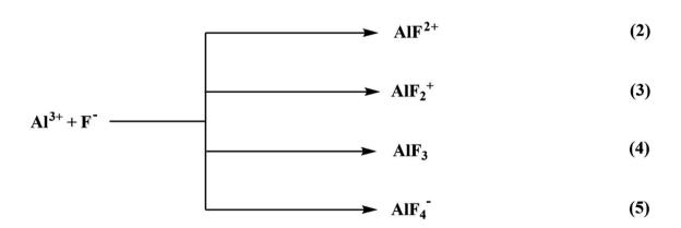
The activated alumina may not be soluble in the aqueous solution comprised of fluoride ions, resulting in the formation of a variety of aluminum and fluoride and hydroxyl-aluminum complexes. The steps of the equilibrium equation to represent the Al–F complexes are as follows:
