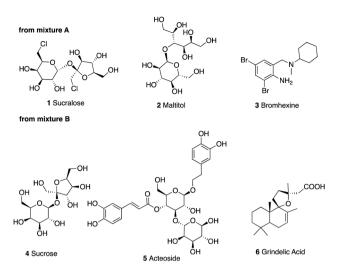
Fig. 6 Main components of mixtures A and B identified by UHPLCaToF.
