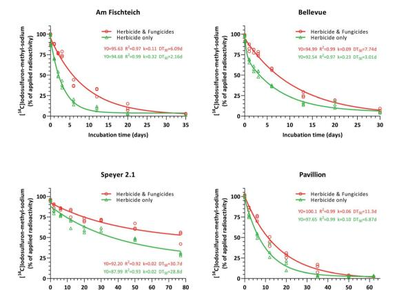
Fig. 4 Recovery (in %AR) of  $[^{14}C]$ -iodosulfuron-methyl-sodium from soil samples (n = 3). Triangular data in green depict soil samples treated with iodosulfuron-methyl-sodium only (controls), circular data in red describe soil samples treated with tebuconazole and prothioconazole 14 days prior to (day -14; dose 1), then on the same day as the herbicide treatment (day 0; dose 2), and again 5 days after application of radiolabeled iodosulfuron-methyl-sodium (day 5; dose 3).
