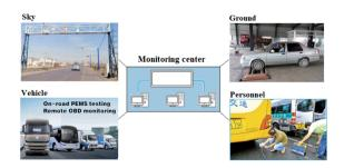
Fig. 1 Integrated vehicle emission monitoring system including sky, ground, vehicle and personnel.
