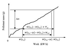
Fig. 7 Schematic diagram of the work-based window method.
