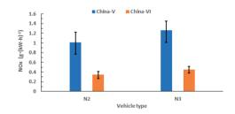
Fig. 4 Specific NOx emissions of heavy-duty diesel vehicles measured by remote OBD.
