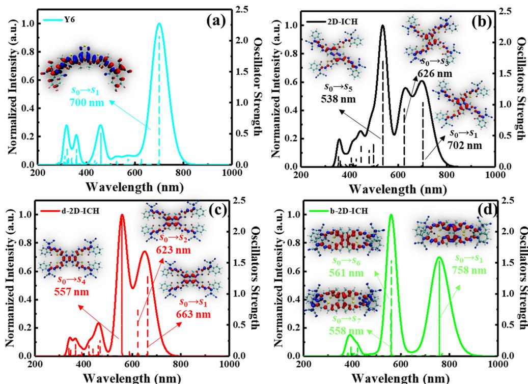
Fig. 5 TDDFT-calculated detailed electron excited states contribute to the absorption spectra of **Y6** (a), **2D-ICH** (b), **d-2D-ICH** (c) and **b-2D-ICH** (d), and the electron (blue) and hole (red) distribution of the excitations with an oscillator strength larger than 0.5 is inserted.
