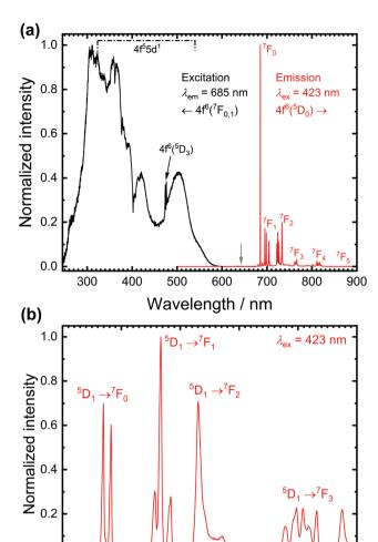
Fig. 1 (a) Photoluminescence excitation (black,  $\lambda_{em}=685$  nm) and emission (red,  $\lambda_{ex}=423$  nm) spectrum of  $SrB_4O_7$ : 0.5%  $Sm^{2+}$  at room temperature. The emission lines are assigned to the  $^5D_0 \rightarrow ^7F_J$  (J=0...6) transitions of  $Sm^{2+}$ . (b) High-resolution spectrum in the spectral range marked with the grey arrow in (a) indicates the presence of weak  $^5D_1 \rightarrow ^7F_J$  transitions.
