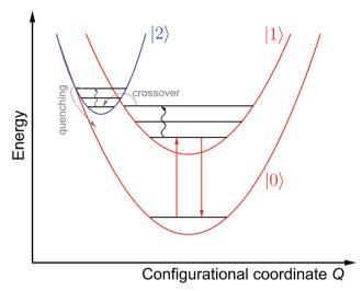
Fig. 3 Schematic overview of the different processes determining the performance of a luminescent crossover thermometer such as Sm<sup>2+</sup> Curvy arrows indicate (multi-)phonon absorption transitions. Note that the excited state |2| has been depicted at lower configurational coordinates to match the theoretical and experimental findings for low excited 4f<sup>n-1</sup>5d<sup>1</sup> states of lanthanoid ions (see also text)
