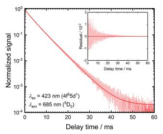
Fig. 2 The photoluminescence decay curve recorded upon monitoring the  $^5D_0 \rightarrow ^7F_0$  transition at 685 nm ( $\lambda_{ex}$  = 423 nm) at room temperature. The solid red line indicates a single exponential fit and the inset depicts the respective residual plot.
