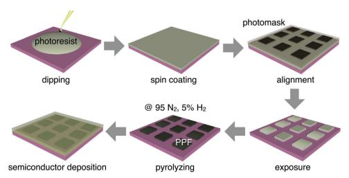
Fig. 1 Schematic drawing of the fabrication process of the patterned PPF electrodes
