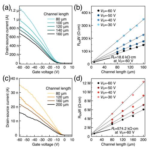
Fig. 5 (a) Transfer I-V of carbon-based OFETs; (b) contact resistance of carbon-based OFETs at various V<sub>G</sub>; (c) transfer I-V of Au-based OFETs; (d) contact resistance of Au-based OFETs at various  $V_{\rm G}$
