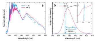
Fig. 3 (a) PLE and PL spectra of  $SrB_4O_7$ : $Eu^{2+}$  microparticles. The PLE spectrum was monitored at 367.2 nm and recorded at 11 and 300 K. (b) PL spectra recorded at 11 K and 300 K excited at 300 nm. In-depth analysis of the ZPL lines and vibronic transitions was presented in ref. 8.
