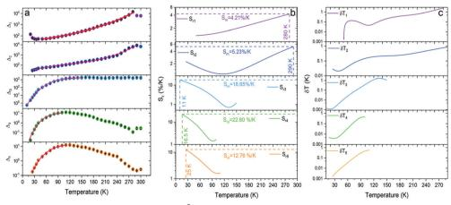
Fig. 7 (a) Thermal evolution of  $\Delta$  parameters for the SrB<sub>4</sub>O<sub>7</sub>:Eu<sup>2+</sup> phosphor, (b) its relative thermal sensitivities, and (c) corresponding temperature uncertainties.
