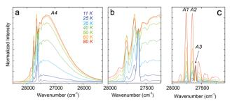
Fig. 6 (a) Temperature-dependent spectra of the  $SrB_4O_7$ : $Eu^{2+}$  material in the T-range of 11–80 K and (b) the magnified part of the A1–A3 lines used for  $\Delta$  parameter determination, (c) presents the spectra after subtracting the broadband fraction related to the 5d  $\rightarrow$  4f transition.
