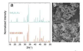
**Fig. 2** (a) X-Ray diffraction pattern of  $SrB_4O_7$  containing 3% of  $Eu^{2+}$  and prepared in an air atmosphere. (b and c) SEM images of the  $SrB_4O_7$ : $Eu^{2+}$  powder, taken at different magnifications (b - 5  $\mu$ m scale bar; c - 2  $\mu$ m scale bar).
