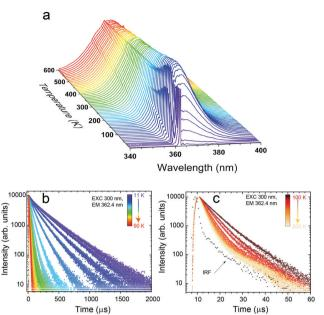
Fig. 4 (a) Normalized (at 362.4 nm) temperature-dependent luminescence spectra of the SrB<sub>4</sub>O<sub>7</sub>:Eu<sup>2+</sup> material, measured in the 11-600 K range upon excitation at 300 nm. Temperature-dependent decay traces of Eu<sup>2+</sup> luminescence, recorded in the range (b) 11-90 K and (c) 100-600 K range.
