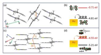
Fig. 5 (a and c) The most favorable plane for charge transfer for (a) TMIQ and (c) TMF4TQ. (b and d) Calculated MO energy level diagram of (b) TMIQ and (d) TMF4TQ upon the Fermi level of gold electrodes.
