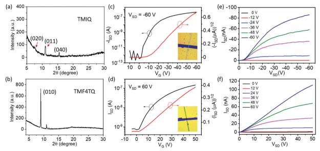
Fig. 4 (a and b) XRD patterns of self-assembled microcrystals for (a) TMIQ and (b) TMF4TQ on OTS-modified SiO<sub>2</sub>/Si substrates. (c and d) Representative transfer and (e and f) output characteristics of OFET devices based on (c and e) TMIQ and (d and f) TMF4TQ micro-ribbons (inset: the corresponding device)
