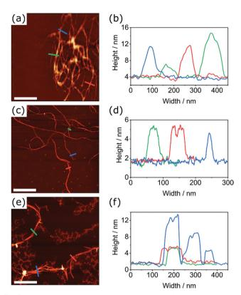
Fig. 3 AFM height images of the morphologies formed by the self-assembly of **PDI1** (a) *cis***PDI1-S4** (c), and *trans***PDI1-S4** (e) in MCH at a concentration of  $5 \times 10^{-5}$  M. Height profiles along each corresponding coloured line, (b, d and f). Scale bars = 1  $\mu$ m.
