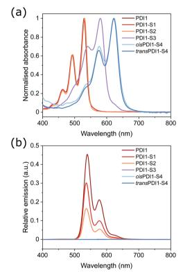
Fig. 1 UV/Vis absorbance spectra (a), and fluorescence spectra (b), of PDI1, PDI1-S1, PDI1-S2, PDI1-S3, cisPDI1-S4, transPDI1-S4, and PDI1-S5. All spectra recorded at a concentration of  $10^{-5}$  M in chloroform. Excitation wavelengths were chosen based on the maxima of the corresponding absorbance; 530 nm for PDI1, PDI1-S1, and PDI1-S2, 580 nm for PDI1-S3, 622 nm for cisPDI1-S4 and transPDI1-S4, and 670 nm for PDI1-S5.
