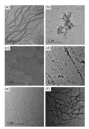
Fig. 2 TEM images of the morphologies formed by the self-assembly of PDI1 (a), PDI1-S1 (b), PDI1-S2 (c), PDI1-S3 (d), cisPDI1-S4 (e), and trans-**PDI1-S4** (f), in MCH at a concentration of  $5 \times 10^{-5}$  M.
