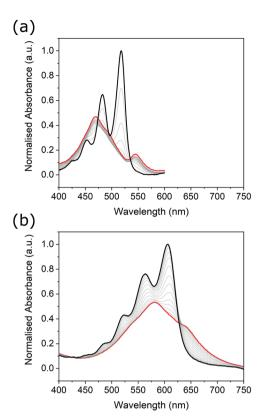
Fig. 4 Changes in the UV/Vis absorbance spectra of PDI1 (a), and trans-PDI1-S4 (b), upon heating from 293 K (red profiles) to 373 K (black profiles) in 5 K intervals. Spectra recorded at a concentration of 5  $\times\,10^{-6}$  M in MCH.
