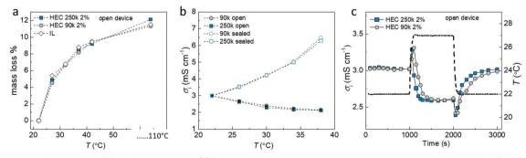
Fig. 3 Temperature dependence of electrolyte properties. (a) Relative mass loss at elevated temperatures due to water evaporation from electrolytes of different compositions (HEC 250k 2 wt%, HEC 90k 2 wt% and without HEC). (b) The saturated conductivity of IL-HEC (250k) and IL-HEC (90k) at different temperatures. (c) The conductivity of electrolytes with HEC 250k and HEC 90k changes with time when temperature increased and decreased.
