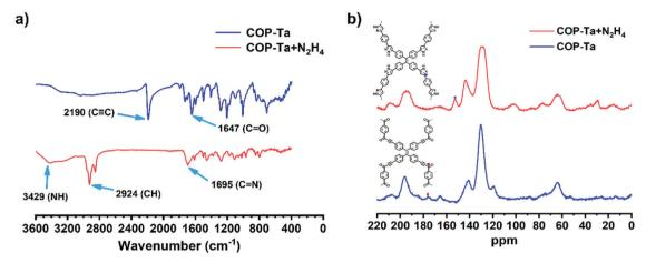
Fig. 7 (a) FT-IR spectra and (b) solid-state <sup>13</sup>C CP-MAS NMR of COP-Ta with (red) and without (blue) the addition of hydrazine.
