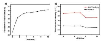
Fig. 4 (a) Time-dependent fluorescence changes of COP-Ta upon the addition of hydrazine ( $\lambda_{ex}$  = 365 nm). (b) The effect of pH on the fluorescence intensity of COP-Ta with (red) and without (black) the addition of 100  $\mu$ M of hydrazine ( $\lambda_{ex}$  = 365 nm).
