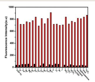
Fig. 5 Comparison of the fluorescence intensity of COP-Ta in the presence of various interfering components (100 µM) in water before (black bar) and after (red bar) the addition of hydrazine (200 mM).
