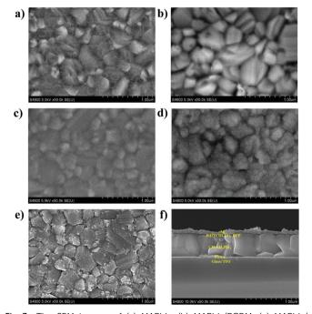
Fig. 3 The SEM images of (a) MAPbI<sub>3</sub>, (b) MAPbI<sub>3</sub>/PCBM, (c) MAPbI<sub>3</sub>/ P(DTCDI-T), (d) MAPbI<sub>3</sub>/P(DTCDI-2T), (e) MAPbI<sub>3</sub>/P(DTCDI-3T) and (f) cross-section of ITO/PTAA/MAPbI<sub>3</sub>/P(DTCDI-2T)/BCP/Ag.
