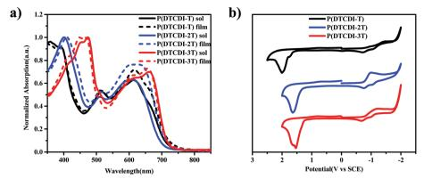
Fig. 1 (a) Optical absorption spectra of P(DTCDI-T), P(DTCDI-2T) and P(DTCDI-3T). (b) Cyclic voltammograms of P(DTCDI-T), P(DTCDI-2T) and P(DTCDI-3T) thin films measured in 0.1 M  $\rm Bu_4N^+PF_6^-$  acetonitrile solution with a scan rate of 100 mV s<sup>-1</sup>.
