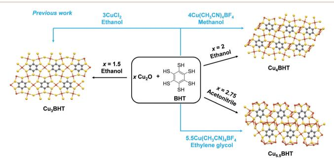
Fig. 1 Comparison of the synthetic methods of  $Cu_xBHT$  (x = 3, 4, and 5.5). The schematic synthesis of  $Cu_xBHT$  using different metal sources and reaction solvents. The previously reported pathways (ref. 13 and 16) are indicated by blue lines and text.
