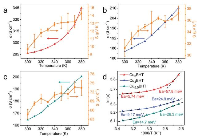
Fig. 3 The charge transport properties of Cu<sub>x</sub>BHT. (a-c) Curves of the variable-temperature electrical conductivity and Seebeck coefficient of Cu<sub>3</sub>BHT,  $Cu_4BHT$  and  $Cu_{5.5}BHT$ , respectively. (d) Plots of  $\ln \sigma(T)$  versus 1000/T of  $Cu_xBHT$ .
