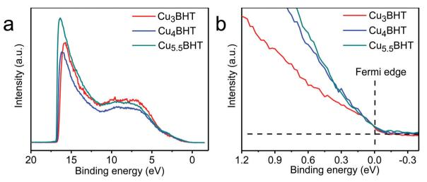
Fig. 4 The UPS analysis of Cu<sub>x</sub>BHT acquired at 300 K. The full spectra and the Fermi edge are shown in (a) and (b), respectively
