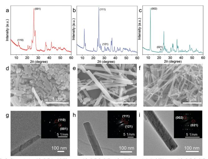
Fig. 2 Characterization of  $Cu_xBHT$ . (a-c) PXRD patterns of  $Cu_3BHT$ ,  $Cu_4BHT$  and  $Cu_{55}BHT$ , respectively. (d-f) SEM images of  $Cu_3BHT$ ,  $Cu_4BHT$  and Cu<sub>5.5</sub>BHT, respectively. (g-i) TEM images of Cu<sub>3</sub>BHT, Cu<sub>4</sub>BHT and Cu<sub>5.5</sub>BHT, respectively. Insets correspond to SAED patterns.
