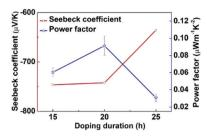
**Fig. 6** Seebeck coefficients and power factors of PBN-TP films exposed to TDAE vapor for different time periods.
