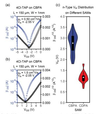
Fig. 5 (a) Transfer I–V curves for the best performing OFET of 4Cl-TAP on CBPA with a drain voltage of -5.0 V for p-channel; (b) transfer I-V curves for the same OFET with a drain voltage of 5.0 V for n-channel; (c) distribution of threshold voltage values for the n-channel OFETs of 4Cl-TAP on CBPA- and CDPA-modified AlO<sub>x</sub> (the white rhombus indicates the average value and the black bar indicates the interquatile range of the data)
