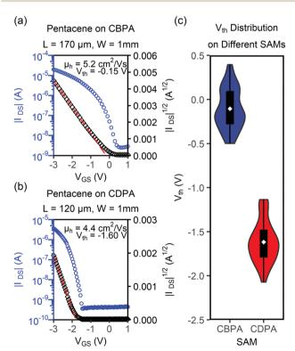
Fig. 4 (a) Transfer I-V curves for the OFET of pentacene on CBPA with the highest field effect mobility; (b) transfer I-V curves for the OFET of pentacene on CDPA with the highest field effect mobility; (c) distribution of threshold voltage values for the OFETs of pentacene on CBPA- and CDPA-modified AlOx the white rhombus indicates the average value and the black bar indicates the interquatile range of the data.
