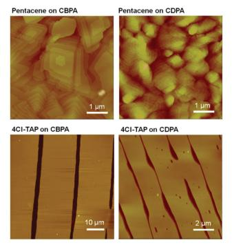
**Fig. 3** AFM images of pentacene films vacuum-deposited on CBPA- and CDPA-modified AlO<sub>x</sub>substrates and 4Cl-TAP films dip-coated on CBPA- and CDPA-modified AlO<sub>x</sub>.
