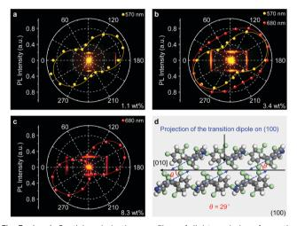
Fig. 3 (a-c) Spatial polarization profiles of light emission from the  $\alpha H$ -PyBTM microcrystal doped with (a) 1.1 wt%, (b) 3.4 wt%, (c) 8.3 wt% PyBTM. The plotted data were fitted with a sinusoidal function. (d) Schematic depiction of the spatial relationship between the  $\alpha H$ -PyBTM molecular transition dipole moment (blue arrows) and the growth direction (black arrow) on the photoexcited plane of the microplate.
