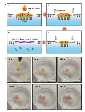
Fig. 1 Principle and process for the formation of 2DCCPs via spaceconfined drop-casting, taking P3HT as an example. (a) Schematic diagram of space-confined drop-casting method. (b) Growth process of 2DCCPs on the surface of water observed with the naked eyes at different times. Scale bar: 2 cm.
